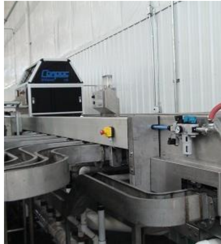
ComPac Fruit Sorting Machine sorts 42,000 cherries/hr
