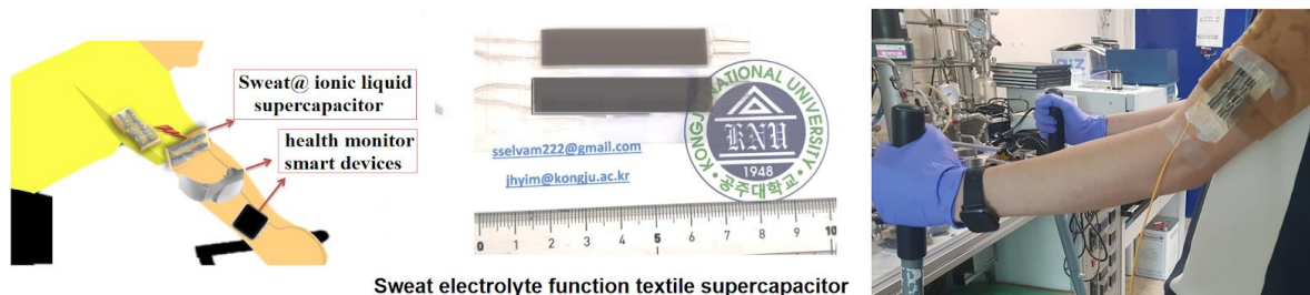
Figure 1: Schematic representation of sweat electrolyte on textile supercapacitor
