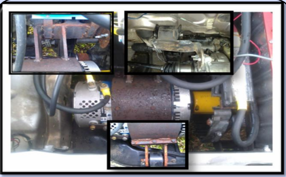
Engine replaced with electric motor, petrol with batteries
