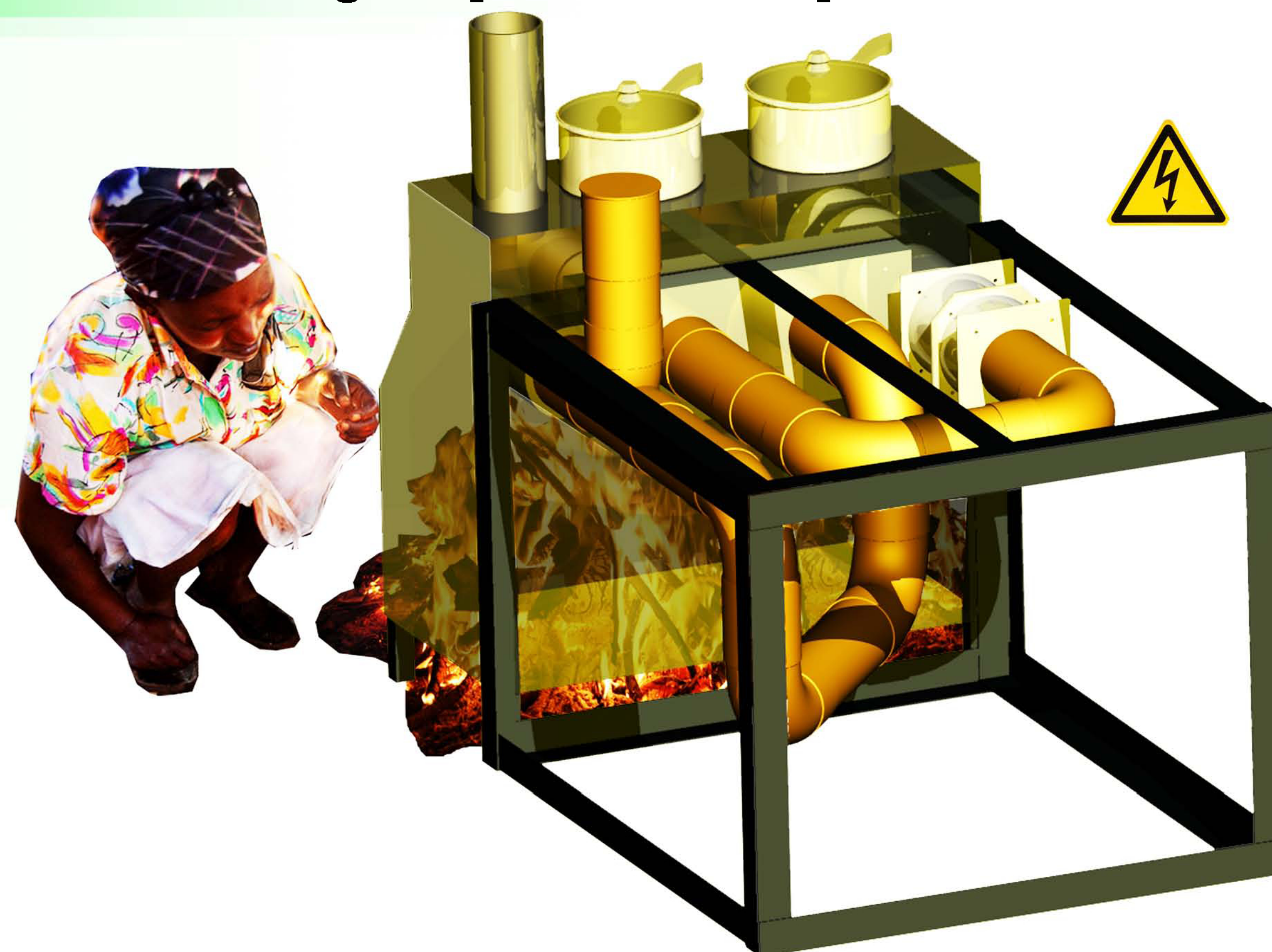
Fig. 2: A Thermoacoustic Stove-Engine for cooking and generating electricity
