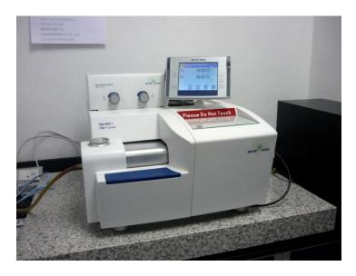
Thermogravimetry (TGA) is a technique that measures the change in weight of a sample as it is heated, cooled or held at constant temperature. Its main use is to characterize materials with regard to their composition. Application areas include plastics, elastomers and thermosets, mineral compounds and ceramics as well as a wide range of analyses in the chemical and pharmaceutical industries.
