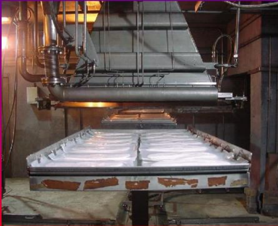
Passing through electron beam for 25 kGy dose.
