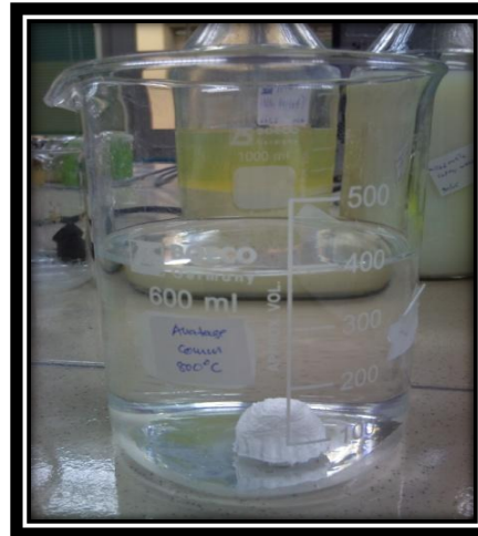
Our geopolymer undergoes leaching test for long term durability
