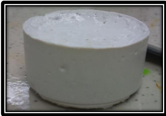
Our geopolymer incorporated with nano alumina for heat insulator and fire proof materials
